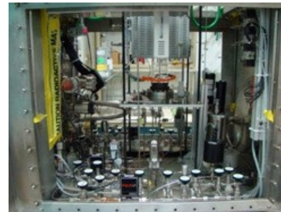
Tritium Gas Absorption Permeation (TGAP)
