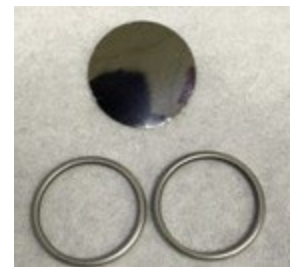
20mm OD specimen and Au wire O-rings (left) and C-rings (right)
