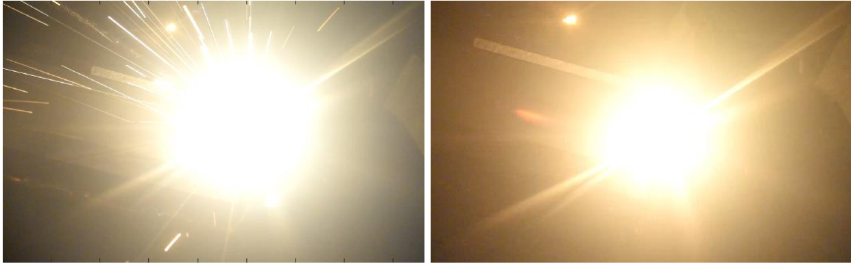
Figure 6: Visible light images from the e-beam hitting the sample surface. Left: Sparks flying off the WHA is an indication of the surface material being ejected during the exposure. Right: Whereas in contrast, when the e-beam hits the pure tungsten surface only the lens flaring from the bright exposure is observed.
