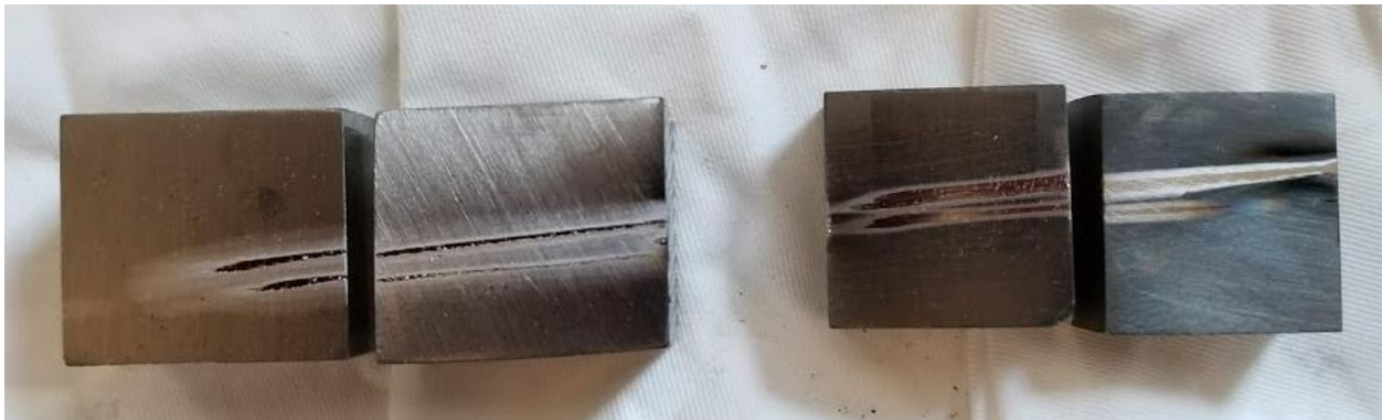
Figure 3: Left 2 tiles are WHA and right two tiles are pure tungsten. When exposed to heat fluxes >500 \text{ MW/m}^2 for \sim 50 \text{ ms} . Both materials demonstrated that they would go straight to surface melting. The beam path can clearly be seen across the four tiles.
