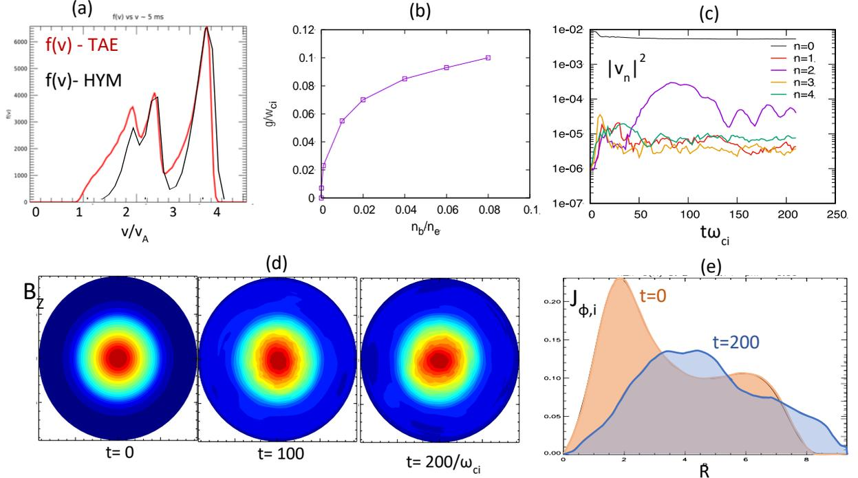
FIG 1. a) Beam ion energy distribution from equilibrium fit (red) and HYM (black); (b) growth rate of  $n=2$  mode vs normalized beam ion density; Nonlinear simulations of FRC for  $S^*=3.6$  with kinetic thermal and beam ions: (c) time evolution of  $n=0-4$  Fourier harmonics of perturbed velocity, (d) contour plots of axial magnetic field, (e) change in the radial profile of the ion current.
