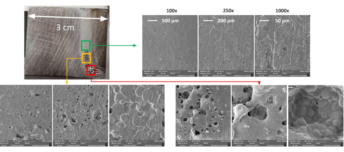
e-beam appears to have passed over the bottom of the sample twice leading to some differential melt/material loss behavior on sample
