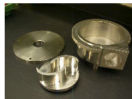
Pump impeller and volute
