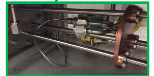
Three cryogenically cooled barrels inside the guard vacuum
