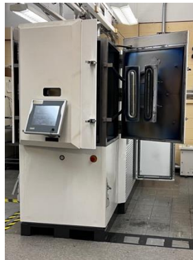
Industrial scale PVD system with multi-targets for depositing HEA materials (alloys, carbides, nitrides, etc.) coatings with wide range of compositions
