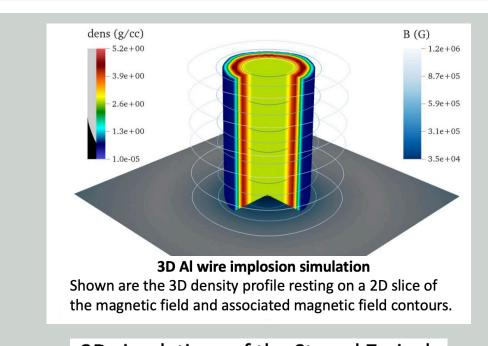
3D simulations of the Staged Z-pinch continue under MIFTI funding.
