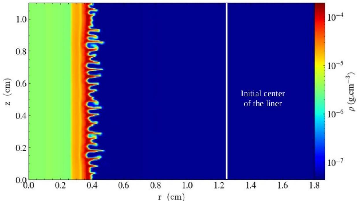
Figure 4. Density map of a 2D FLASH simulation of Conti et al. [43] experiments, taken at  $t = 95$  ns, for a convergence ratio of 3.
