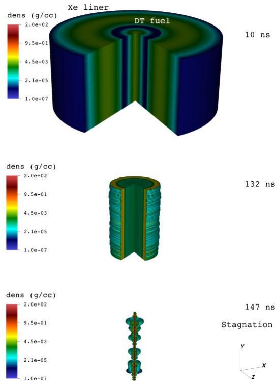
Figure 8. A sample 2D FLASH SZP1\* simulation. Shown is the evolution of the density profile and the MRTI development, rendered in three dimensions by utilizing the cylindrical symmetry of the simulation.
