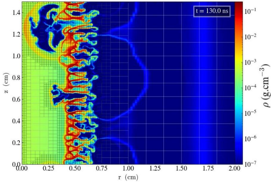
Figure 7. Density map of a high resolution (0.02 mm) SZP1\* simulation at  $t = 130$  ns. RTI growth is so important that, in the non-linear phase, the bubbles destroy the liner-target interface.
