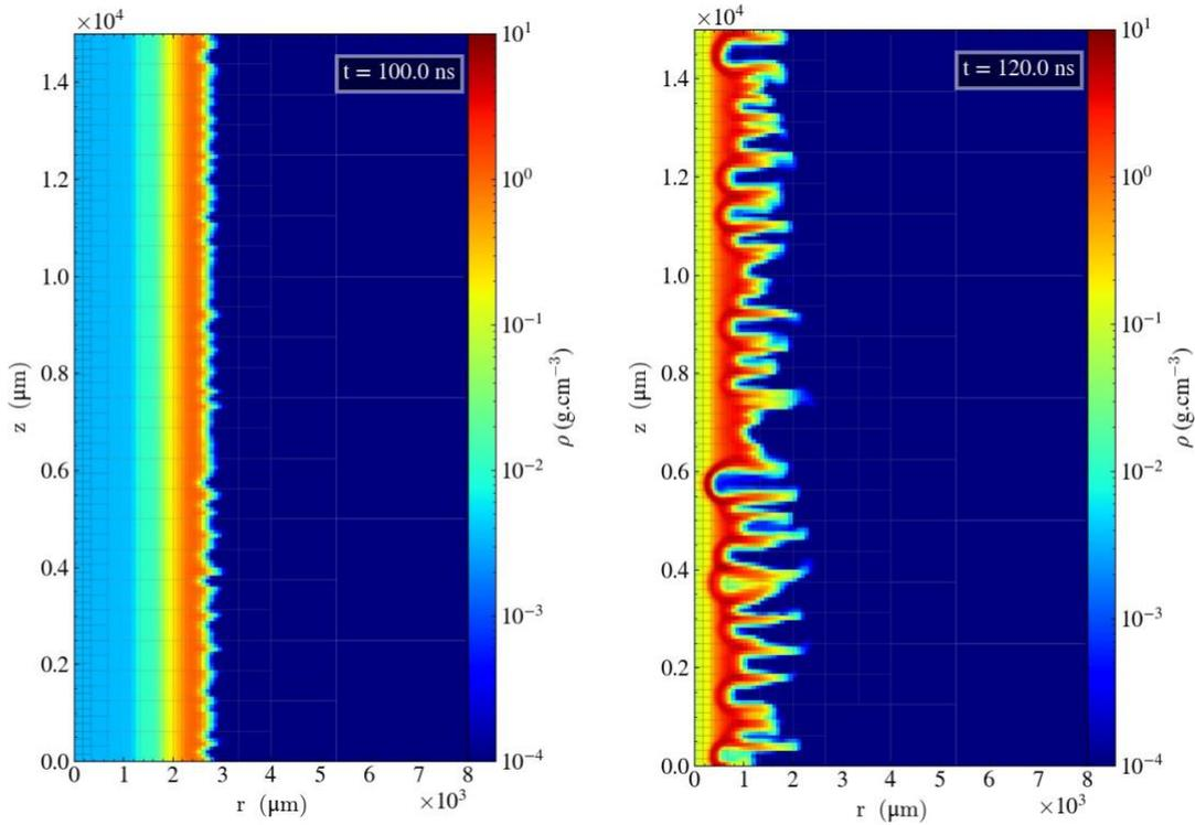
Figure 6. Density maps of a SZP1 simulation at  $t = 100$  ns and  $t = 120$  ns. RTI growth is particularly important in this setup which could degrade the implosion.
