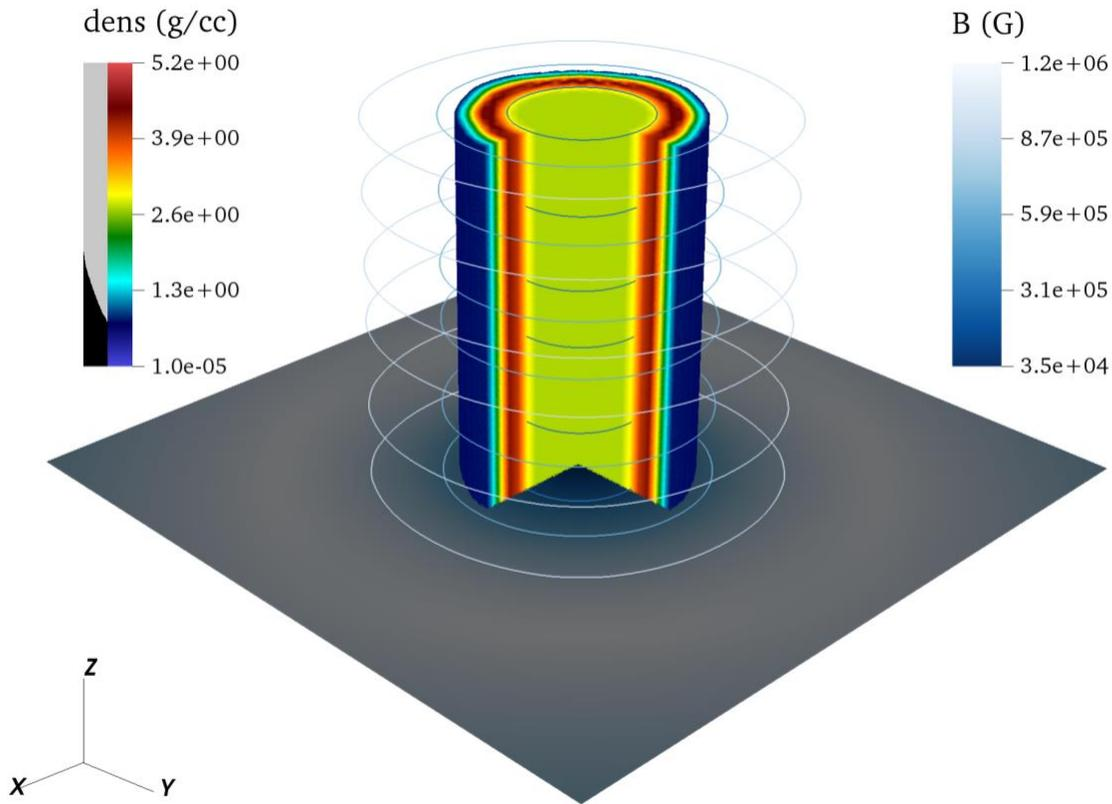
Figure 10. 3D Al wire implosion with FLASH. This is the first 3D Z-pinch simulation with the FLASH code. Shown are the 3D density profile resting on a 2D slice of the magnetic field and associated magnetic field contours.
