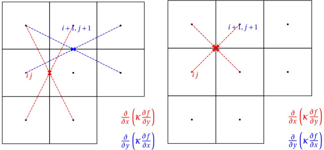
Figure 9. Stencil dependence for the different collocations of the derivatives along x (red) and y (blue) for the face-centered (left) and edge-centered (right) cases.
