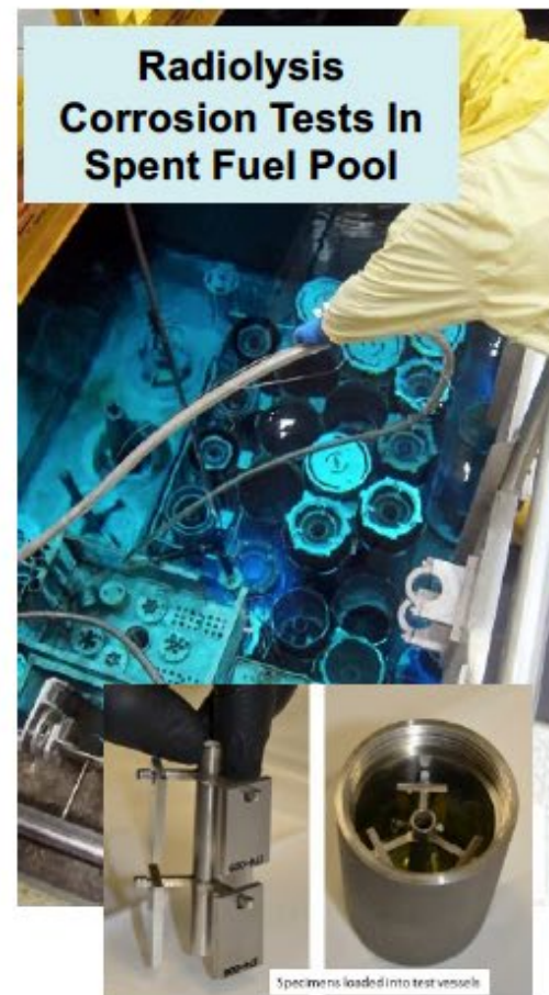
Specimens loaded into test vessels
