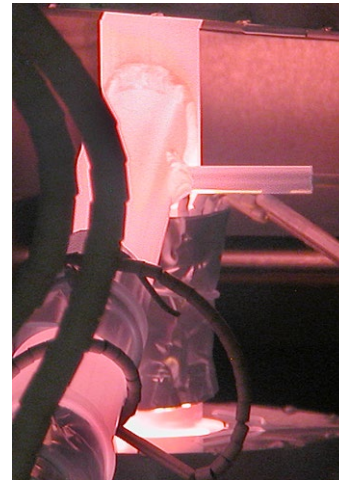
V-4Cr-4Ti Li loop at 700°C through chamber viewport
