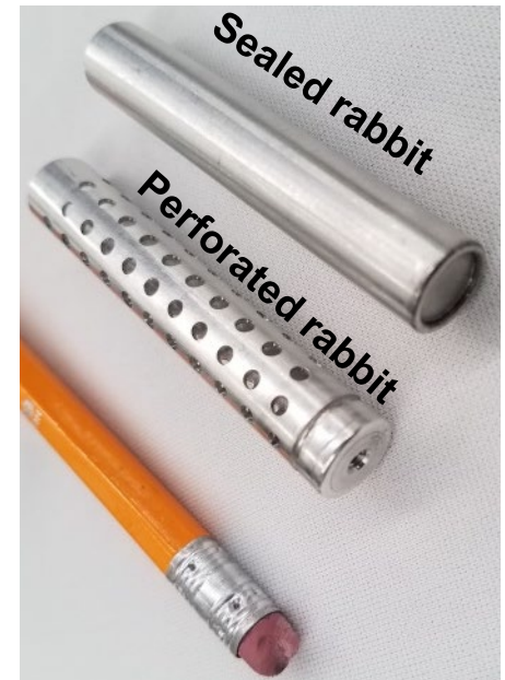
Rabbits inside target rod holder
