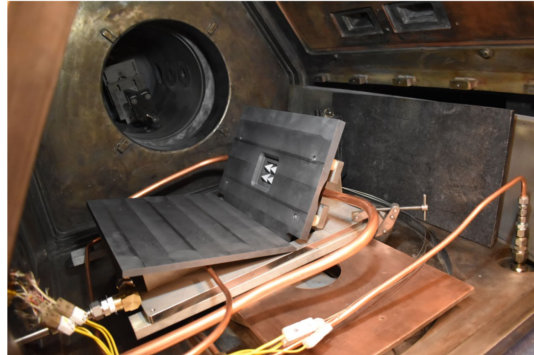
Electron Beam (EB) Facility at ARL-PSU with MPEX Microwave Absorber Test Article
