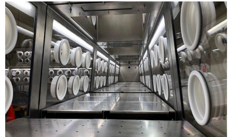
Glovebox interior provide abundant space to test individual tritium processing components as well as integrated systems testing
