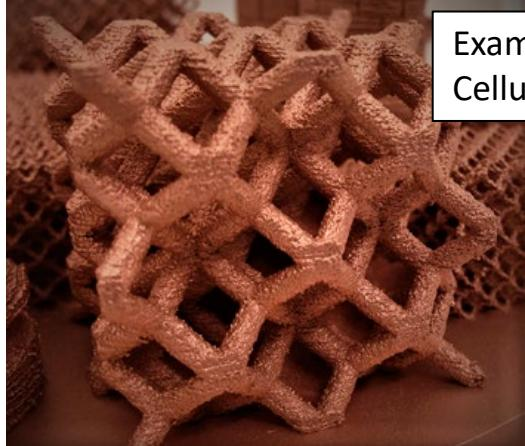
Example of Additively Manufactured (AM) Cellular Structure for Hydride Bed Heat Transfer
