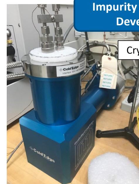
Cryocooler With Sample Loaded
