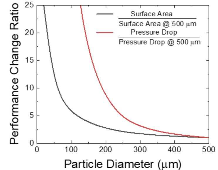
Performance versus particle diameter of packed column containing 500 μm particles as a baseline
