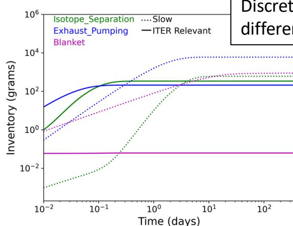
Discrete-time model calculated Inventories for different sub-system processing times
