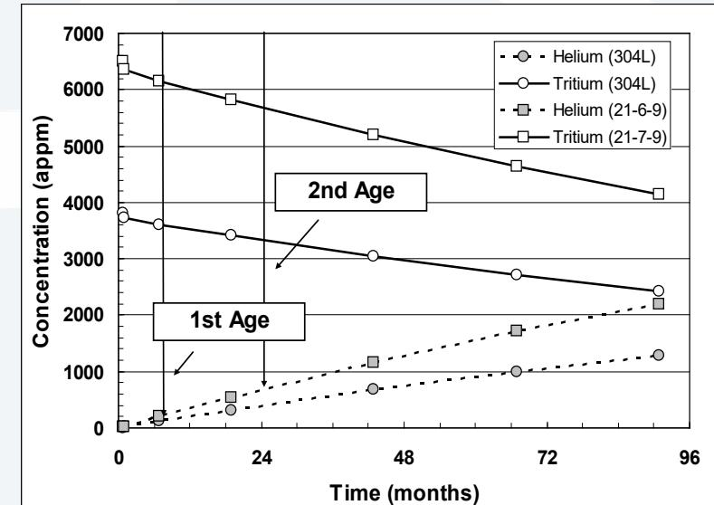
Hydrogen/Tritium Exposure at elevated temperature and pressure followed by low temperature aging to build-in helium Without Losing Tritium.
