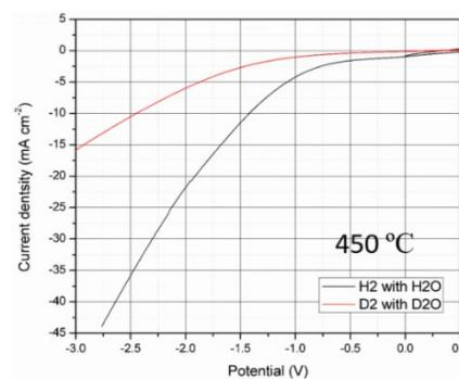
Figure 2. IV curve of graphene coated BCZYYb at 450 °C.
