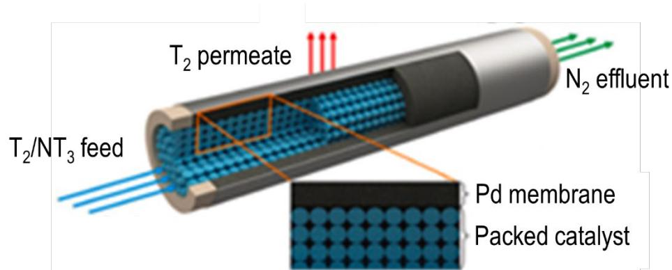
Permeation Membrane Reactor (PMR) Packed With Ammonia Decomposition Catalyst.
