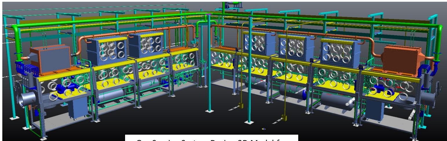
Gas Service System Design 3D Model for an HPDS glovebox system
