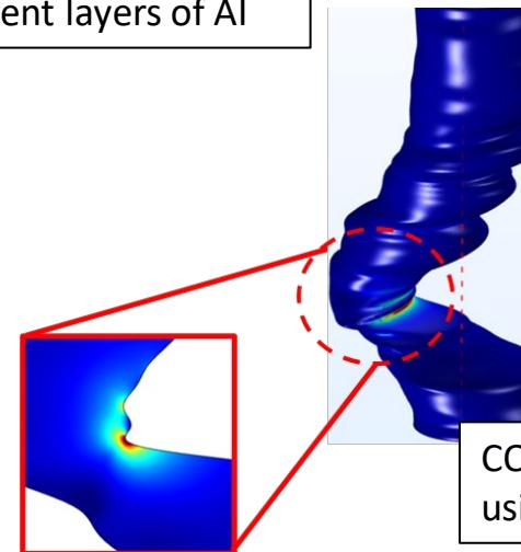
COMSOL stress response of a 3D solid created using the SRNL developed LatticeJ© software
